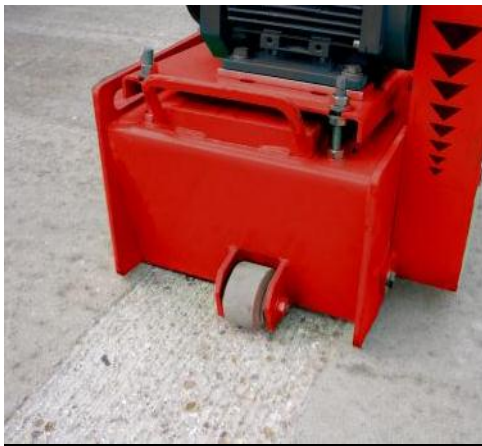
Cleaning & keying concrete
